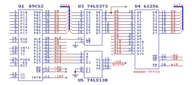
The CH375 has the common passive parallel interface, connects to various MCU, DSP and MCU directly. In common MCS-51 typical application circuit, CH375 can connects to system bus of MCU through 8-bit passive parallel interfaces  $D7 \sim D0$ , -RD, -WR, -CS and A0.
